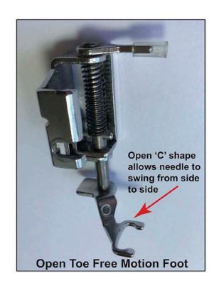
When using the free motion foot, remember to lower the feed dogs and alter the **stitch** length setting on your machine to zero, or as close to zero as it will go.
